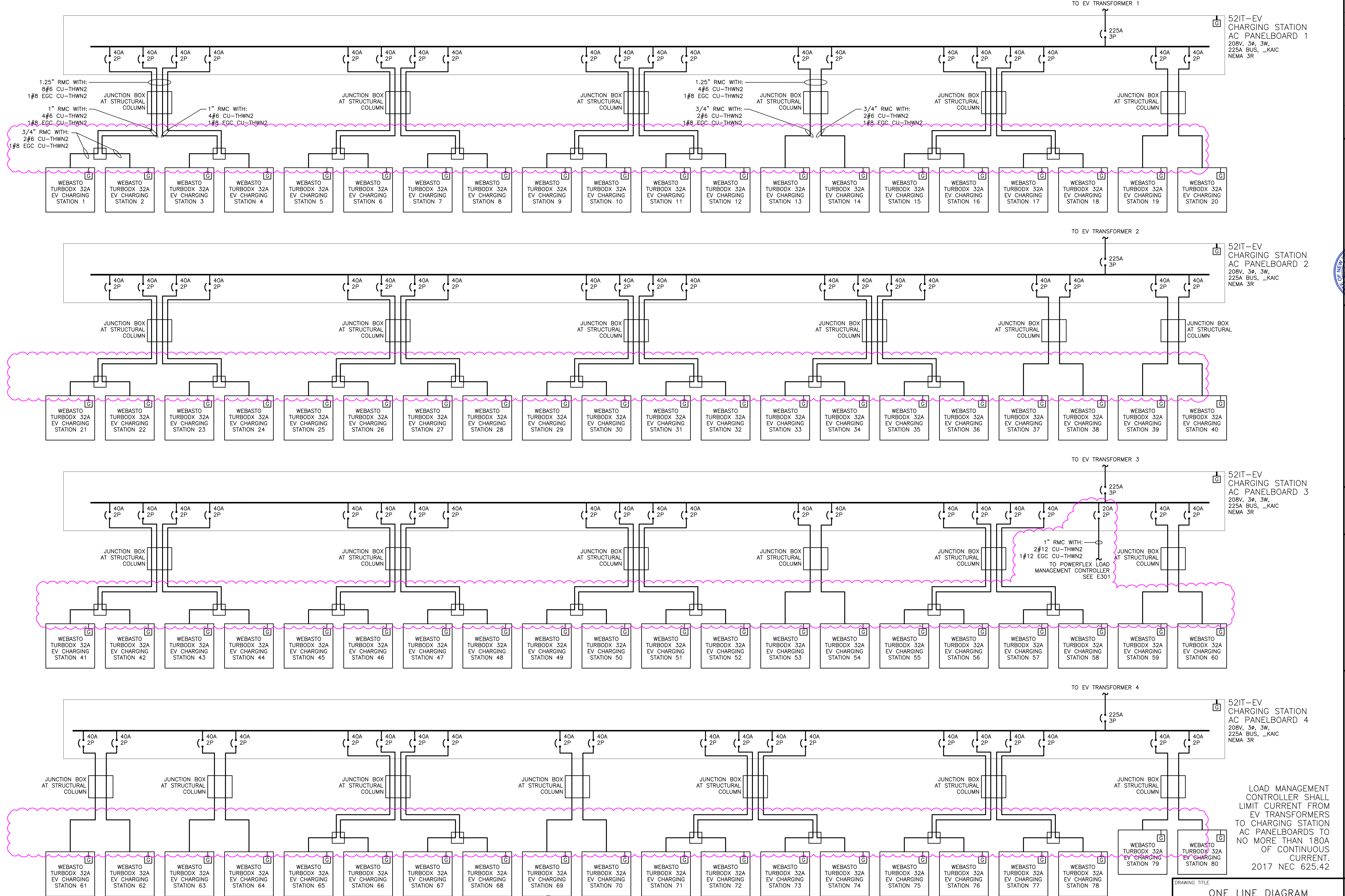
1 ONE LINE DIAGRAM - EV CHARGING E302 SCALE: NONE
