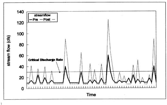
Stormwater management practices limited to no increase in pre-development peak flow rates may not increase the number of runoff events that exceed critical erosion velocity but will increase the duration of each such event that does occur. Stormwater management methods that minimize the adverse effects of development could be emphasized in the regulations and their application vigorously pursued by the permitting authorities.
