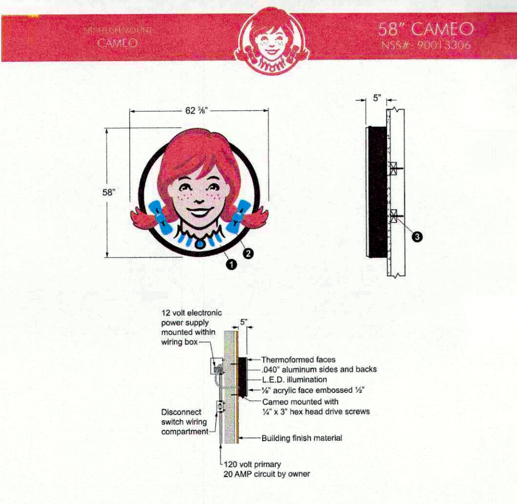
FLUSH MOUNTED 58" WENDY'S CAMEO SIGN DETAIL
