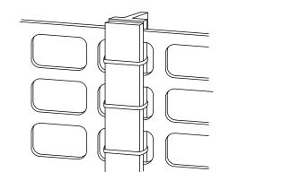
INSTALLATION INSTRUCTIONS 1. T-Post should be placed a maximum of 10 feet apart 2. Vertical Strand of fence should be sandwiched between flat side of T-Post and 1"x2" wood slat 3. Wire Ties or plastic cable ties can then be used to secure 2. Fence should be tensioned by hand only the slat and fence strand to the T-Post.
