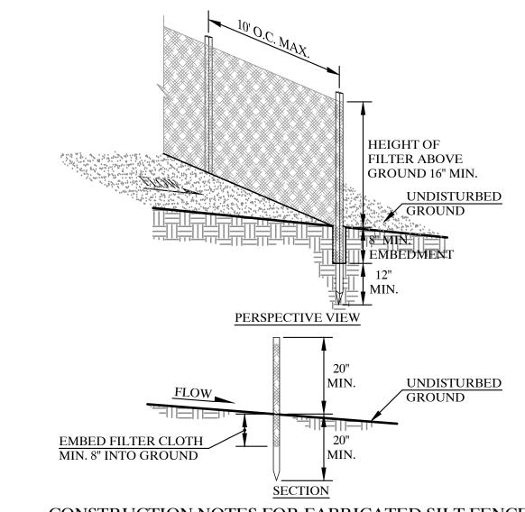
CONSTRUCTION NOTES FOR FABRICATED SILT FENCE 1. FILTER CLOTH TO BE FASTENED SECURELY TO POSTS: STEEL EITHER T OR U TYPE OR 2" HARDWOOD POSTS AT TOP AND MID SECTION.
