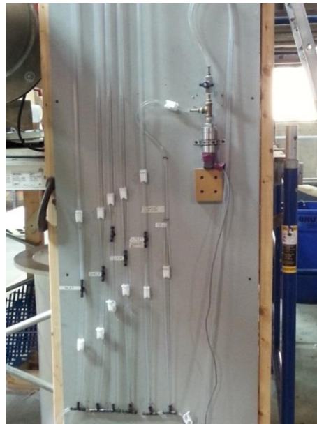
Figure 6 Pressure Measurement Instrumentation
