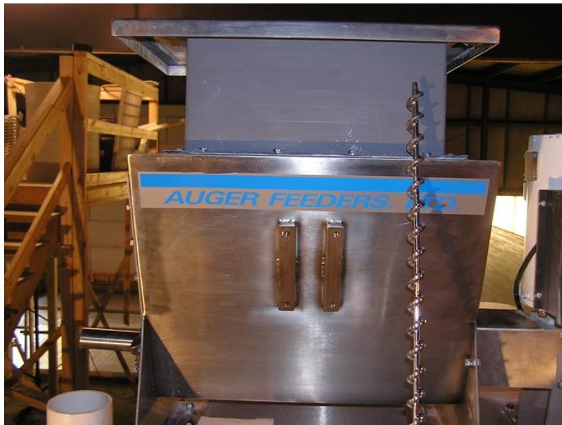
Figure 7 Photograph Showing Variable-Speed Auger Feeder
