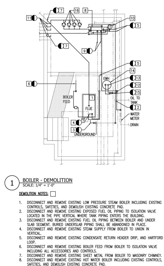
9. DISCONNECT AND REMOVE EXISTING HOT WATER SUPPLY PIPING FROM BOILER TO POINT INDICATED, INCLUDING FLOW CONTROL VALVE.
