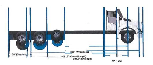
Item #1: One New Combination Single Engine Hydro Excavation Machine with Positive Displacement Vacuum System Mounted on a Heavy Duty Truck Chassis or Equivalent.
