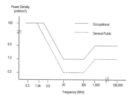
Because the FCC's RF exposure limits are frequency-shaped, the exact MPE limits applicable to the instant situation depend on the frequency range used by the systems of interest.
