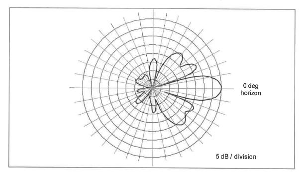
Figure 1. 1900 MHz Directional Panel Antenna – Vertical-plane Pattern
