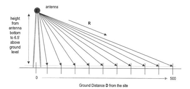
Figure 2. Street-level MPE% Calculation Geometry
