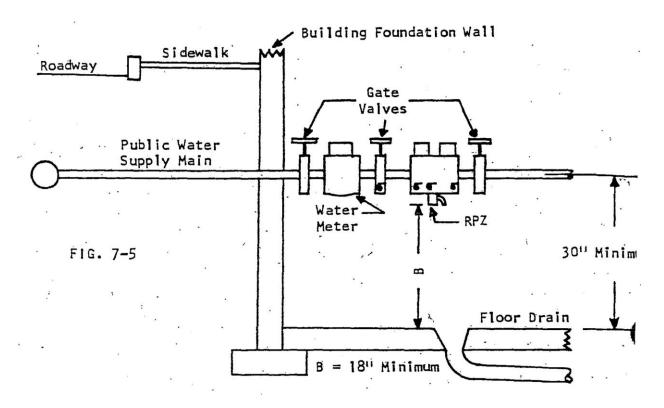
NOTE: Device to be installed above highest possible flooding.
